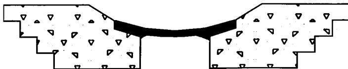
Architectural Joint Design in "U" Configuration, also with Recess for Flush Installation
