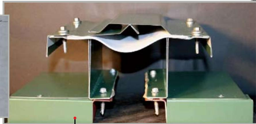
Figure 3: A mock-up of a metal roof expansion joint using precured silicone sealant along with metal cover plates. Photo courtesy of Building Research Systems Inc.
