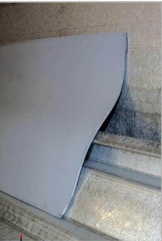
• **Figure 4: A mock-up of a roof-to-wall transition application using precured silicone sealant**
