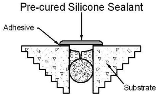
Fig. 2: Repair joint
