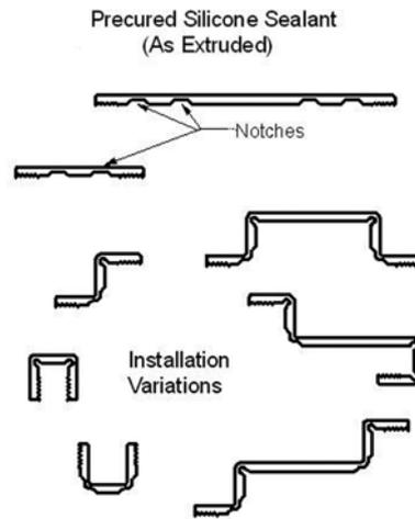
Fig. 6: Installation variations of notched precured silicone sealant
