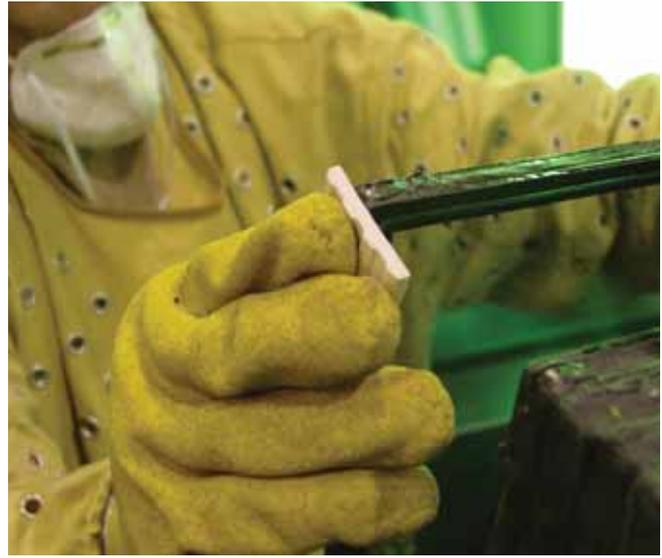
**A pre-cured sealant pad being used for tooling of a hot-melt butyl IG sealant.**
